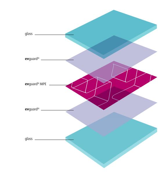
Folienwerk Wolfen GmbH also offers a PET-MPE film ("100 % modified copolyester"). In combination with the **ev**guard<sup>®</sup>, **ev**guard<sup>®</sup> MPE establishes an additional advantage in terms of stability, durability, shear modulus effect and printability. **ev**guard<sup>®</sup> and **ev**guard<sup>®</sup> MPE can be processed by using the existing suggested cycle times for normal lamination.
